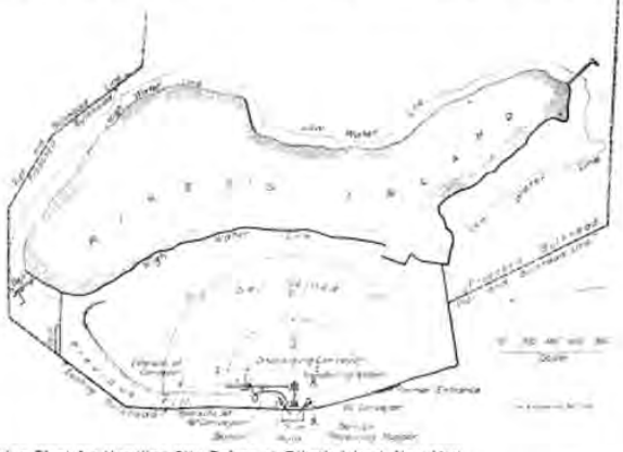
General Arrangement of Conveying Plant for Handling City Refuse at Riker's Island, New York.
